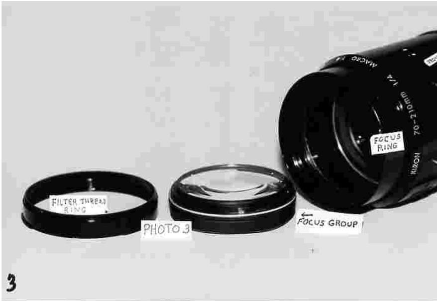
When they can be reached, completely remove the three set screws. Normally, I avoid completely removing set screws because they are tricky to reinstall, but the points of these press into fine threads and if left in place will damage the threads.
