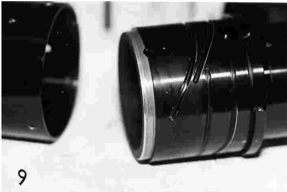
Some burrs were found on the inner sides of the holes for the Fat Plastic Set Screws and elsewhere some polish of the black anodizing suggested binding. The Inner Zoom Ring was pulled back and taped to the Lens Barrel to keep the glass back. Then the old grease and some aluminum shreds were
