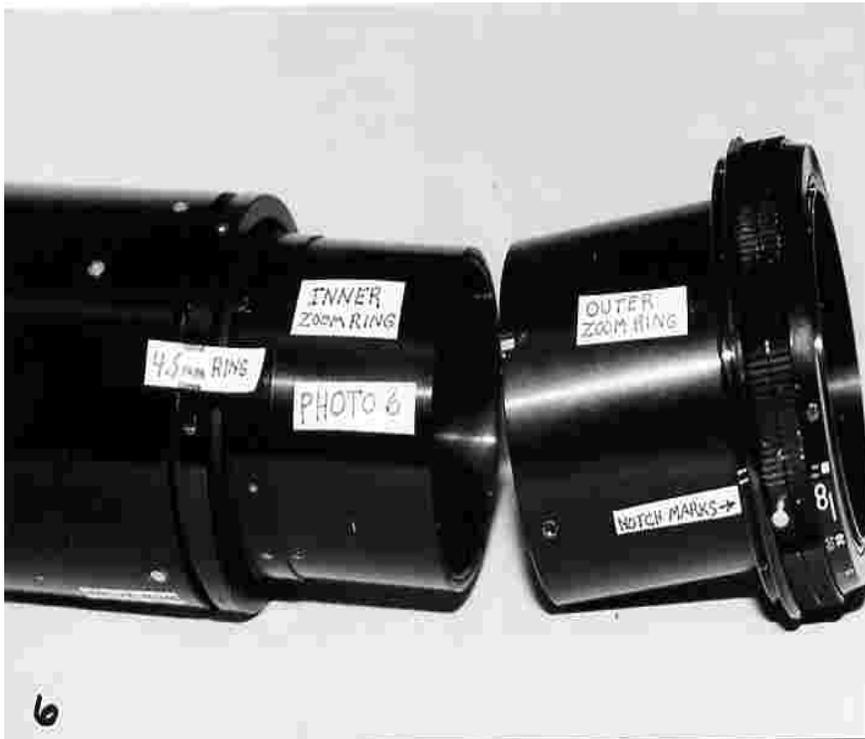
There is only one square notch on the front of the Outer Zoom Ring. It fits over the only notch in the Inner Zoom Ring which was out of sight under the outer ring in *PHOTO 4*. These notches provide alignment for reassembly.
