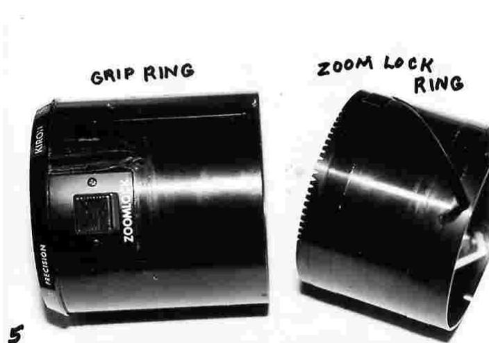
so. Mark the notch on the Zoom Lock Ring that is closest to the marked notch on the Grip Ring. Either at this time or later during reassembly the Zoom Lock Ring may be removed from the Grip Ring (the set screws will interfere if not loosened enough) for cleaning and lubrication. *PHOTO 5* shows the Zoom Lock Ring removed from inside the Grip Ring.
