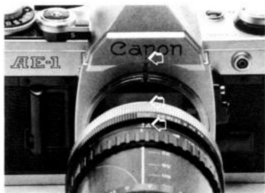
Lens shown is Kiron 35-135mm. Mounting procedure is the same.
