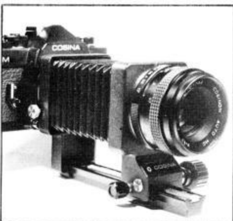
This is a manual bellows focusing unit fitted with the camera's standard lens. The lens would be used in the manual mode — turning the aperture ring to fully open for viewing and focusing, then manually stopping down to the f/stop required for the picture before the shutter is released.
