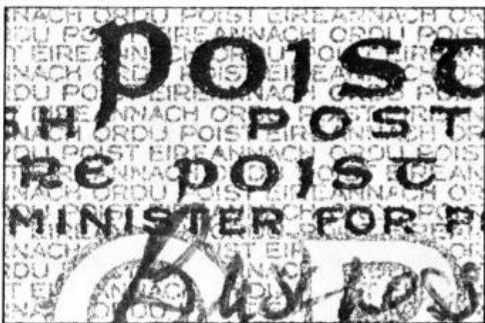
Using the macro attachment set on its lowest magnification together with a +3 close up attachment, image quality is degraded, but by comparison with the results obtained using the close-up lenses alone, we can see a marked improvement.
