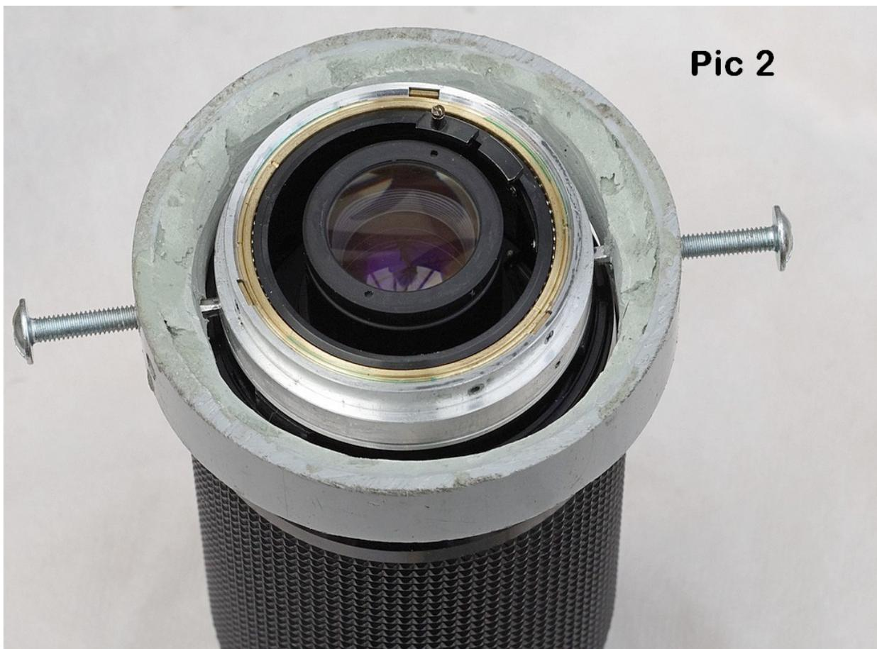
8. Prime lens assembly (rear optical group + iris) is held in by 3 x round head JIS. The rear optical group unscrews from the iris assembly, loosen this while it is still in the lens.
